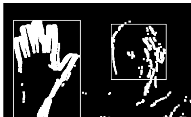
Figure 2: Motion islands of a user performing a swipe while moving his upper body
