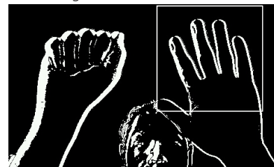
Figure 3: The result of using an absdiff classifier trained on open hands. Note that the head and fist are not detected
